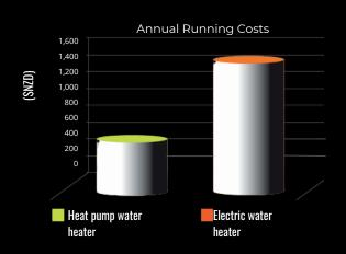
\*Estimation based on IWH280L STC's in Zone 3 under medium load, obtained from independent laboratory test results and followed by TRNSYS modelling and a retail electricity cost of \$0.30c per kWh.
